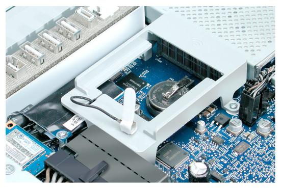
4. Slide the AirPort Extreme card into the slot until it clicks into place. Connect the AirPort antenna cable to the AirPort Extreme card.
